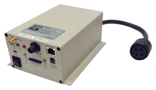
The *Model 395* is our smallest data logger at 0.68 kg (1.5 lb) and comes with 2 GB of internal data storage. Minimal power consumption (2.5 watts) allows for ≈20 days of life at 100 amp-hr with one 12 VDC battery. The *Model 395* can be used for fixed surveys in a stand-alone kit with option for remote access via optional cell modem/WiFi.
