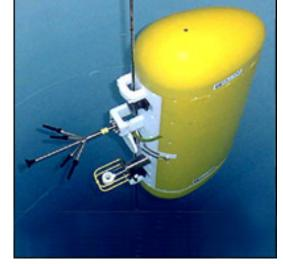
The MMP follows a programmed trajectory along a mooring cable, automatically sampling the water column with a suite of
