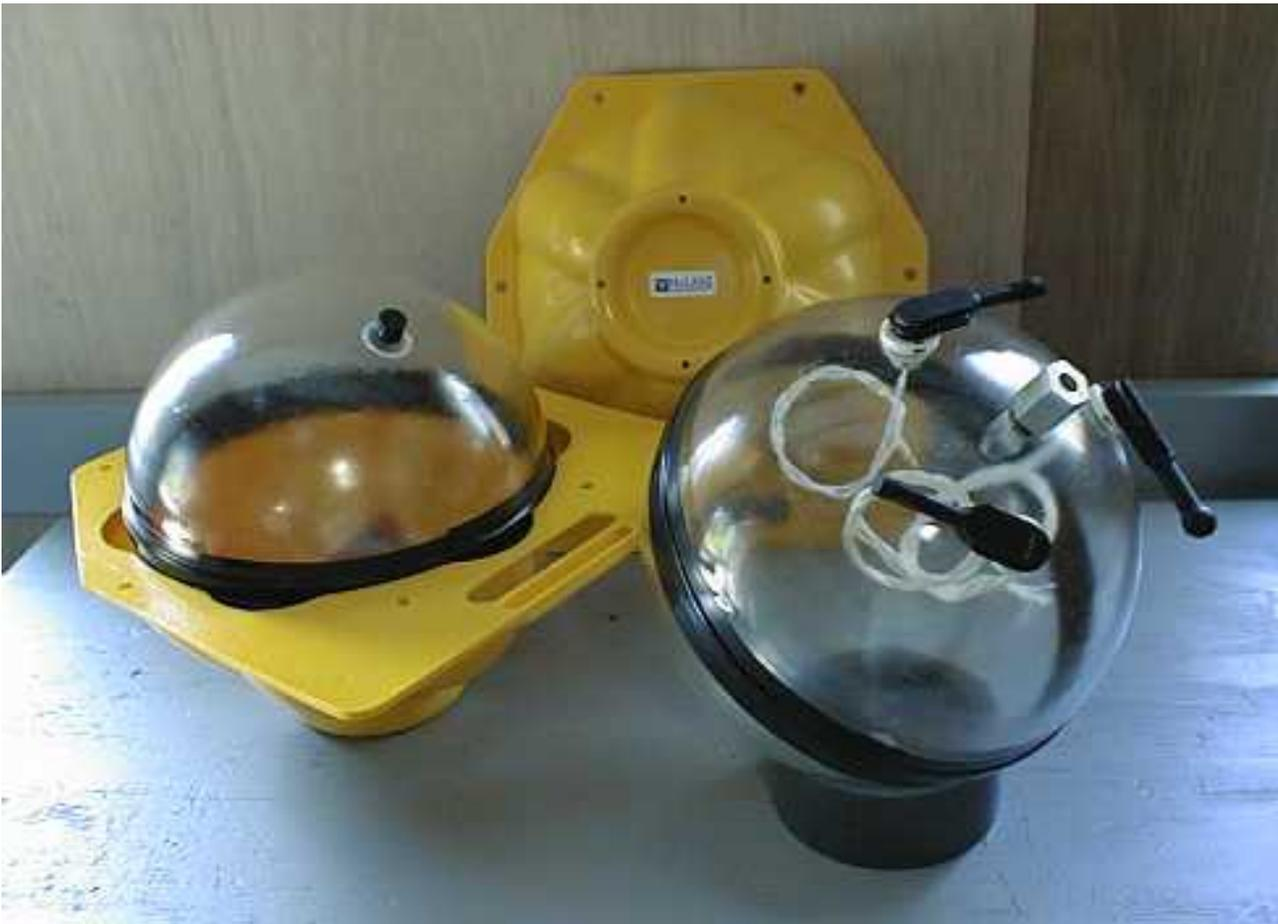
On the left is a G2200 instrument housing with a vacuum port placed 30 degrees from the pole of the sphere. On the right is a custom housing built for Woods Hole Oceanographic Institution. The penetrators on the top hemisphere include three multi-pin electrical connectors spaced 120 degrees apart along a circle located 30 degrees from the pole and a titanium hydraulic feed-through located at the pole. A vacuum port is installed in the matching hemisphere.
