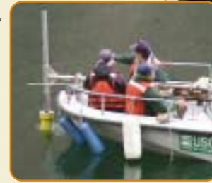
The Argonaut-SL can be mounted on a single bank of an open channel and profile 2-D water velocity in a horizontal sampling volume extending across the channel cross-section.
