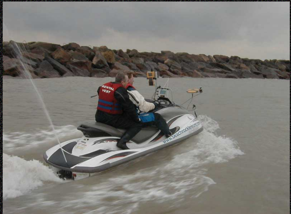
JetSki system surveying in East Anglia
