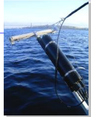
ISUS Nitrate sensor mounted on T-frame.
